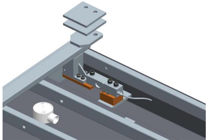
NOTE: use cable ties through existing holes under the steelwork to attach cable and junction box assembly.
